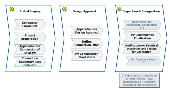
Figure 2 - Connection Process
