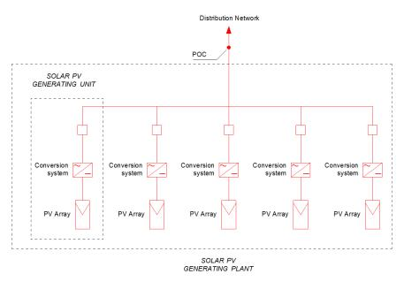
**Solar PV Plant Voltage** - Unless stated otherwise, voltage refers to the root-mean-square value of phase-to-phase voltages.
